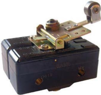
The MICRO SWITCH™ 6AS Series consists of two large premium BZ/BA/BM/BE snap-action switches ganged together and actuated by a single actuator. Operating characteristics are dependent upon the type of individual switches and actuators chosen. Field adjustable operating point on one or both basic switches.
