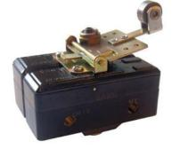
The MICRO SWITCH<sup>™</sup> 6AS Series consists of two large premium BZ/BA/BM/BE snapaction switches ganged together and actuated by a single actuator. Operating characteristics are dependent upon the type of individual switches and actuators chosen. Field adjustable operating point on one or both basic switches.
