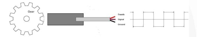
The APM-FREQ detects and measures the frequency of the output from the inductive sensor. The AMP-FREQ maximum frequency is 400Hz therefor consideration must be made when designing the system to ensure that the maximum frequency from the system will not exceed this.
