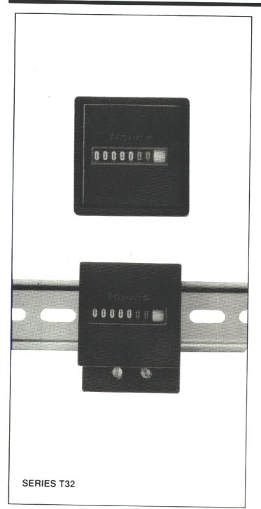
Series T32 is a synchronous motor driven hour meter at AC and stepper motor driven at DC. This hour meter can withstand even the most rugged applications. The completely insulated housing provides substantial protection against environmental influences. Applications include control of the running time of machines, apparatus, and instruments as well as recording maintenance time, warranty time, or rental use time.
