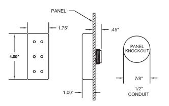
The ATC Diversified Electronics GFD Series is intended for the use on ungrounded systems to detect and indicate the phase of the first ground fault condition. This enables corrective action to avoid the potential hazards resulting from a second ground fault.
