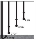
As above, but wired with a high alarm float switch
