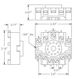
The Model 51X016 11-Pin Socket can be surface or DIN-rail mounted and is suitable for use up to 300 VAC.
