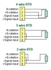
In 4-wire hookup, different pairs of leads are used to apply the excitation current and sense the voltage drop across the RTD, so that the IR drop across the excitation leads is not a factor.
