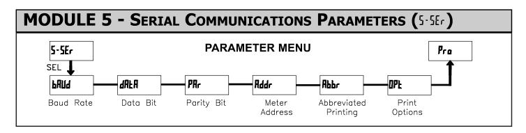
Module 5 is the programming module for the Serial Communications Parameters. These parameters are used to match the serial settings of the CUB5 with those of the host computer or other serial device. The Serial Setup Parameters are only accessible when an optional RS232 or RS485 serial communications module is installed in the meter.
