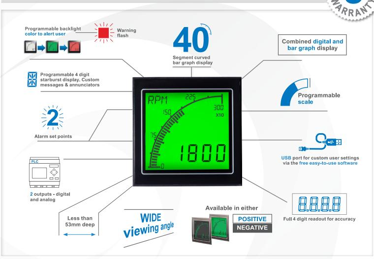
The Advanced Panel Meter (APM) Rate Meter was developed for use in flow applications, production lines and motorspeed monitoring. It combines the instant visual representation of an analog meter with the speed and accuracy of a digital meter. The unique display is viewable in most environmental conditions and features a programmable scale and color changing backlight for instant recognition and precision measurement.
