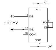
Measuring an input voltage referenced to a floating supply, i.e. the input voltage and the meter's power supply are isolated from each other.
